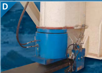
D One of four leveling cylinders rated at 1500 tonnes each (with vertical restraints on the right)
