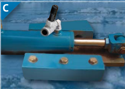
C Typical horizontal restraint to lock the drillfloor/substructure and skidbase during drilling operations
