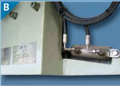
B Actuation cylinder on vertical restraint
