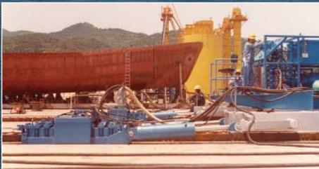
A pair of Gripper Jack Assemblies used to loadout ships of 4,000 tonnes with a roller beam transfer system.
