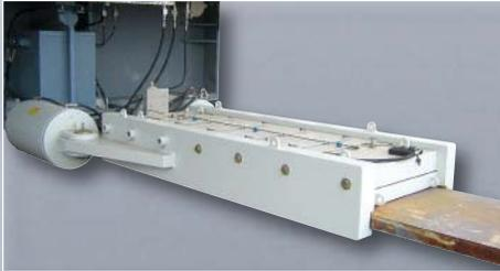
One of two 760 tonne Gripper Jack Assemblies used to skid a skidbase at temperatures down to -39C . The Gripper Jacks also provide horizontal restraint against seismic forces.
