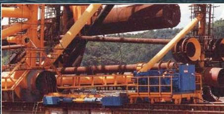
A Jacket Loadout system using multiple gripper jack assemblies to skid a 17,800 tonne offshore jacket.
