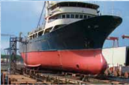
5,000 tonne Shiplift with longitudinal and side transfer system
