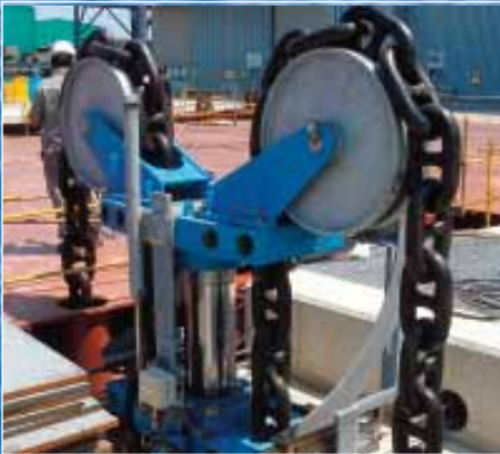
Linear Chain Jack rated for 260 tonne lift capacity
