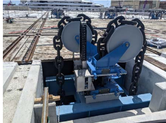
Figure 4 Examples of vertical lifting devices are the shiplift and the OmniLift™ Floater/Maintenance Vessel Launch and Recovery System. A typical lifting component is the chain jack, shown here.
