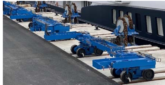
Figure 2 A rail based self-propelled transfer system.
